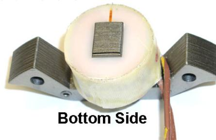
13. Route the wires through the stator plate and sleeving. Then, using the 553-2697 insertion tool, install the pins in the AMP connector plug.
