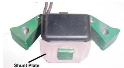
12. Slide the new coil on the stator frame (NOTE: The wires will come out on the side of the coil – not the bottom). Fold the wires towards the outside and route them down and under the frame. If the old coil had shunt plates, you **MUST** use the new shunt plate provided with the new coil. **If the old coil did not use a shunt plate, do NOT install one.** Bend the top frame lamination up and the bottom lamination down to lock the coil on the frame.
