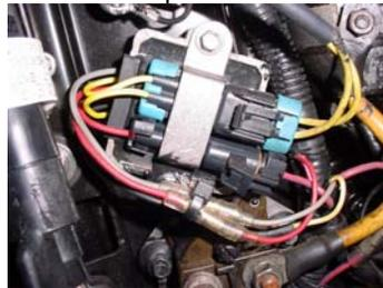
7. On V6 engines, replace the 20 Amp fuse with the 30 Amp fuse supplied per the factory Service Bulletin 2001-09. All 3 of these fuses should be the 30 Amp rating. On all other engines, ignore the 30 Amp fuse supplied as it is not required.
