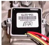
9. Connect all wires to the regulator/rectifier, matching color codes (the gray stripe on the OEM stator can be connected to either yellow wire on the regulator/rectifier).
